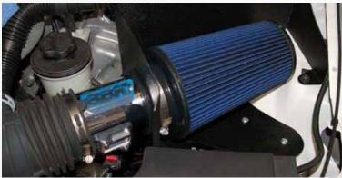
Install Chrome BBK inlet tube into the stock air inlet tube. The Mass Air Sensor should point forward. Plug in the mass air sensor. Install the BBK Air Filter. Tighten all the clamps.
