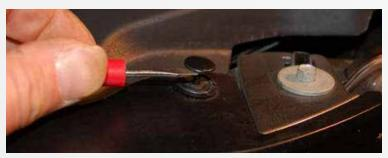
Disconnect the negative battery terminal. Remove the plastic radiator cover by prying up the center of the plastic pin heads at the slots cut on each side. Pull pins out to remove. Lift cover off and set aside.
