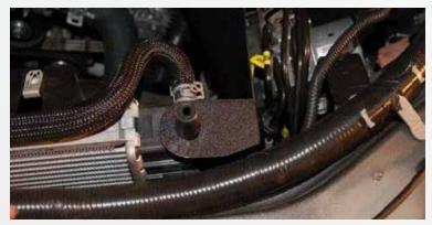
Place the filter shield in place locating the stock grommets back into their original mounting holes and placing front mounting tab over peg of the radiator. Re-install the mount and tighten the bolts. Install and tighten the other stock air box mounting bolt in the filter shield on the inner fender.
