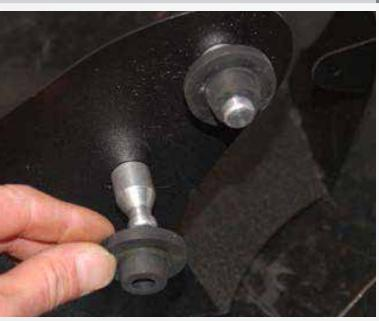
Assemble the 2 supplied aluminum pins to the bottom of the filter shield using the supplied  $\frac{1}{4}$ "-20 x  $\frac{1}{2}$ " Phillips screws. Install the stock rubber grommets to the pins.
